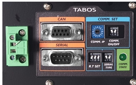
BMU (Battery Monitoring Unit)
